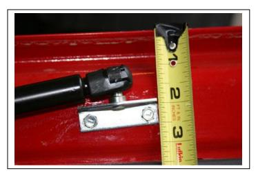
the bracket with the slanted spring. Go ahead and drive in both screws, using the supplied star washers.
