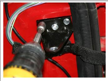
5. Snap the rod end of the gas spring onto the tub mounted ball stud bracket and then open the tailgate all the way till it stops so you can position the small, tailgate bracket. You will be installing the tailgate side ball stud bracket so that the spring pushes the tailgate all the way to the Jeep hinges' built-in stop.
