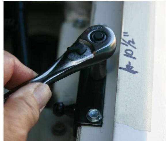
4. Now the hood. Place a ball stud bracket per the photo, 1 7/8" in from the edge of the hood with the ball stud lining up with the 27" mark on the tape on the hood; ball stud facing out. Put a star lock washer on a self-drilling sheet metal screw and drive it through one of the holes in the bracket as you did with the fender bracket. Do the same for the other hole in the bracket. Hand-tighten the screws with your 5/16" socket just as you did before behind careful not to strip out the holes.
