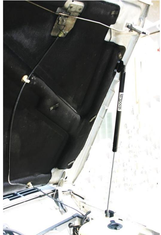
7. Have your second gas spring handy, then have a friend hold up the hood or brace it open with something and take down the Jeep's prop rod. It has to be removed or it will be in the way of the gas spring in its parked position. Using your 10mm socket, extension and ratchet wrench, remove the two bolts holding it on, per the photo. Remove it and put it in your parts collection in case you ever need it in the future. Finish installing your gas spring, remove the tape and you are done!
