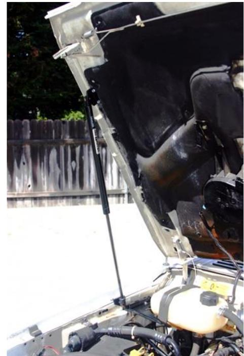
If you ever have to remove a gas spring, slip a small screwdriver under the small semi-circular clip near the end and lift it up to release it from the ball stud it is capturing. To replace a gas spring, just snap it back onto the ball stud.
