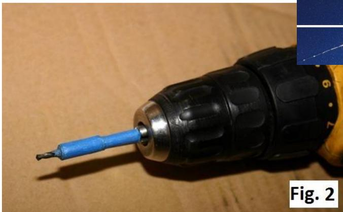
Wrap some masking tape around your 7/64" drill bit as shown in **Fig. 2** so it will only go approx. 1/4" through the sheet metal. This is to prevent you from drilling too far and damaging anything that may be below the surface of the sheet metal. Make certain the tape is wrapped tight and that it goes all the way to the drill chuck so the tape doesn't slide. Take a
