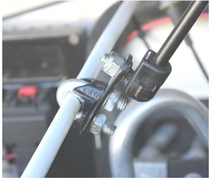
**Remember!** They are U-bolts and almost all u-bolts seem to stretch and loosen as they conform whatever they are wrapped around. So go back and re-tighten them after a week or so.
