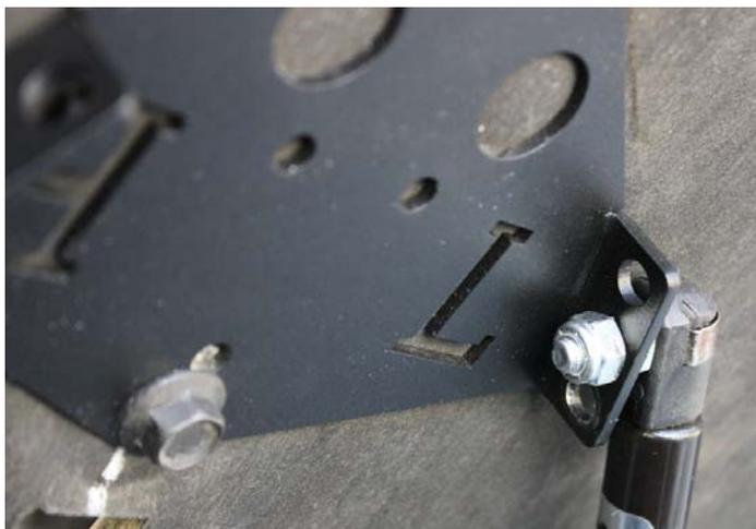
Install driver's side ball stud in middle hole.
