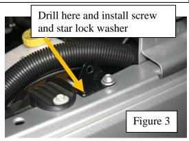
lower Ball Stud Bracket to the Jeep. If you use an electric drill and a nut Driver, set it on a low speed and go slowly to almost snug, then hand-tighten with a 5/16" socket and ratchet wrench. Be careful to not break the screw. If it's going in too hard, ream the hole out slightly with the drill.
