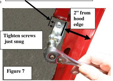
part of the gas spring should be up. Upside-down gas springs also have a shorter life than properly installed ones.
